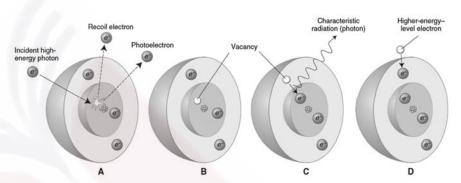
An incident electron (A) ejects an electron from an inner orbital creating a photoelectron, a recoil electron, and an electron vacancy (B). C, An electron from an outer orbital fills this vacancy, and a photon is emitted with energy equal to the difference in energy levels between the two orbitals. D, Electrons from various orbitals may be involved, giving rise to other characteristic photons. The energies of the photons released are characteristic of the target atom.
