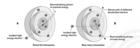
Bremsstrahlung radiation is produced by the direct hit of an electron on a nucleus in the target (A) or, much more frequently, by the passage of an electron near a nucleus, which results in electrons being deflected and decelerated (B).
